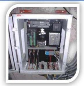
SISPL Vibrating Wire Data Logger has been designed to measure up to 16 channels of vibrating wire instrumentation features include IP67 Rating, Stand Alone System, Multiple Power Options, RS232 Communications Interface, Up to 8 Input Channels, Over 1000 Scans Available, Menu Driven User Options, Simple Sensor Connection
