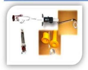
SINGLE POINT MECHANICAL ROD EXTENSOMETERS
