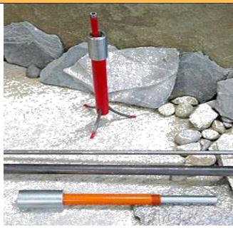
Systel Settlement device are designed to generate settlement profiles within the changes in the relative position of structural elements associated with many types of structure.
