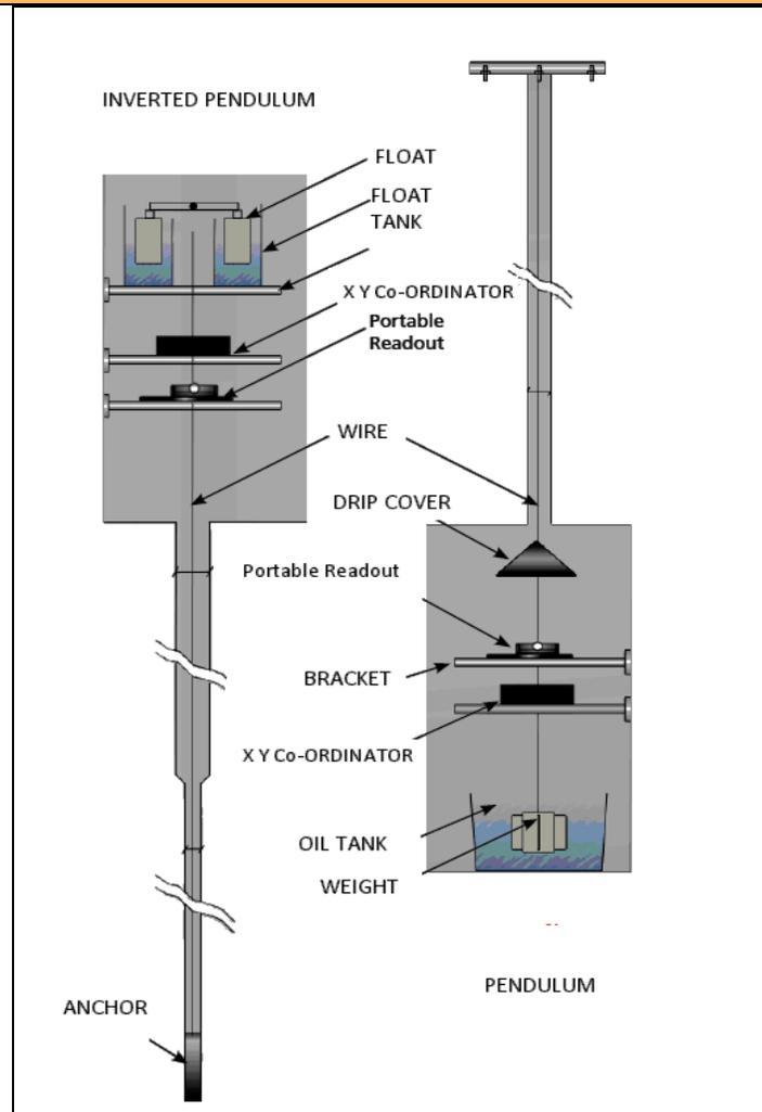
The Pendulum Systems are primary used to provide reliable, accurate long term monitoring of displacements in dams.
