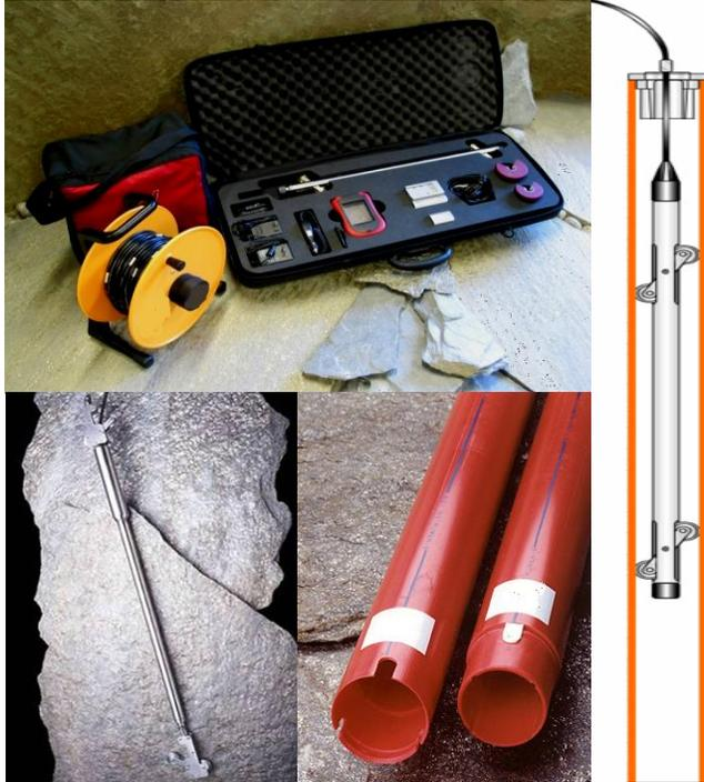
Systel Inclinator Probe is used in conjunction with inclinometer casing for the measurement of lateral earth movements which might occur in unstable slopes, landslides, dam and roadway embankments, and landfills. They are also used to measure deflections in
